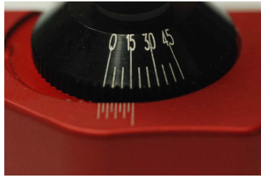
Use 15~20 for Bennet Angle when using the articulator.
