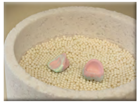
Well-dried result before sintering with YETI SINT
